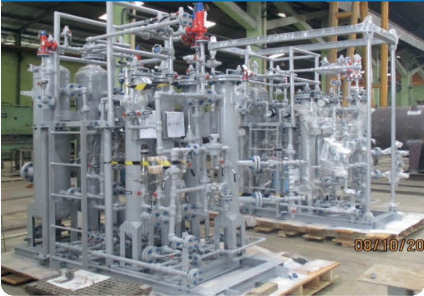
Instrument Gas Dryer Package
