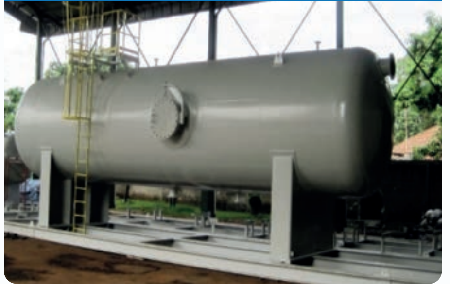
3 PHASE LP SEPARATOR
